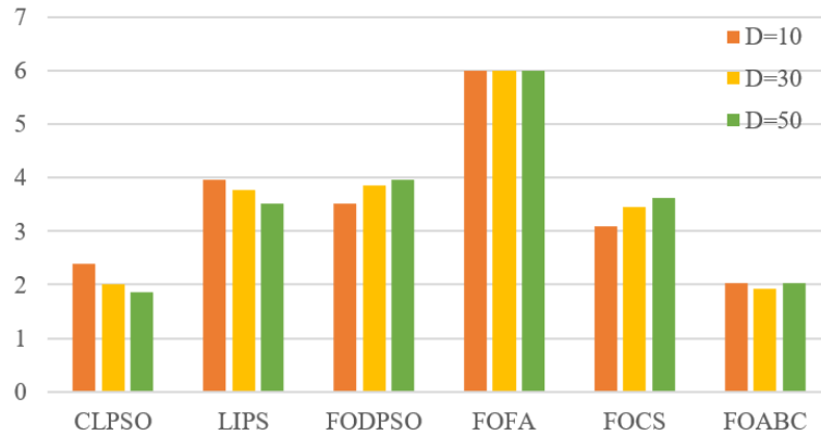
Fig. 5.5. Average rankings of non-ABC algorithms and FOABC by Friedman test with D = 10, 30, and 50
