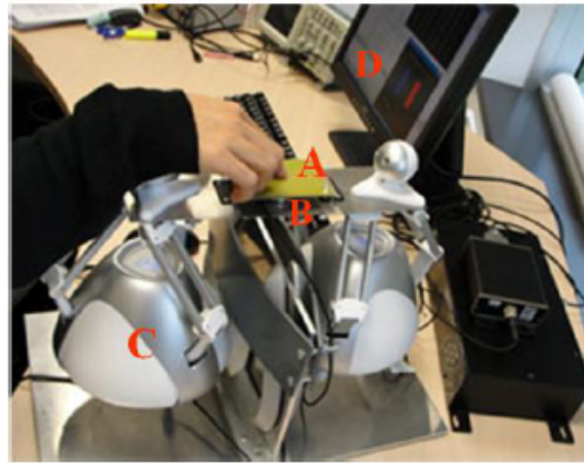
FIGURE 2.9: A 3-DOF haptic interface for spatial texture and shape rendering a) tactile plate, b) force sensor, c) two falcon kinesthetic device, d) control PC [16]
