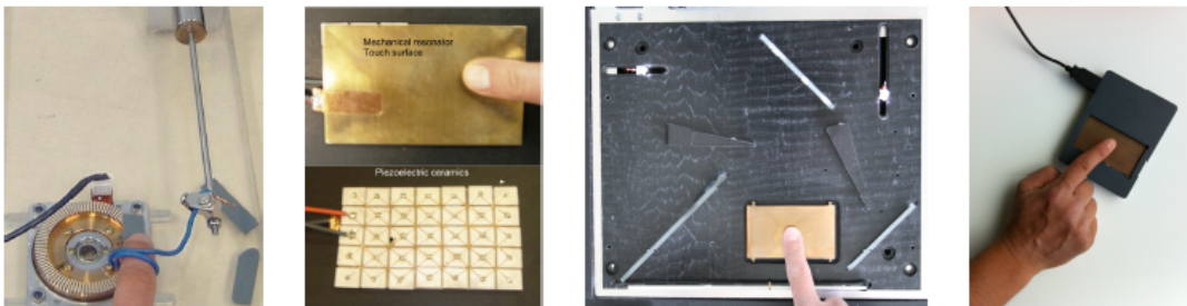
FIGURE 2.18: The evolution of the STIMTAC tactile plate design at L2EP lab. From left to right: 1D prefiguration (2004) with the free stator of a USR60 ultrasonic motor and a ring shaped resonator, 2D feedback (2007) with a tactile plate on top and piezoelectric ceramics at the bottom, 2D input and tactile feedback (2008) and compact standalone USB opaque prototype (2010) [29].
