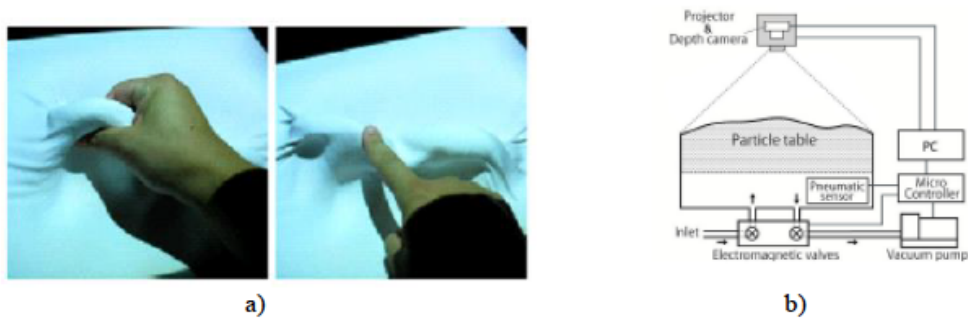
FIGURE 2.4: The ClaytricSurface interactive surface for shape rendering by dynamic flexibility control [10]. a) Surface in a soft state (left) and hard state (right) , b) System hardware
