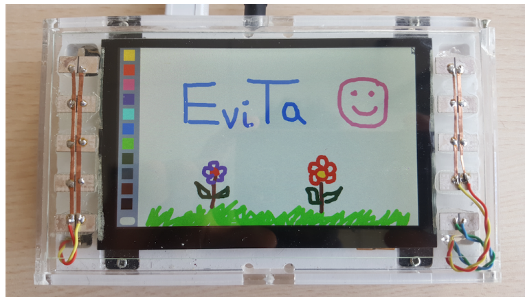
FIGURE 3.18: The setup of the paint application. Each color is associated to a specific texture which allows users to feel and draw at the same time. The white color is served as an eraser tool.
