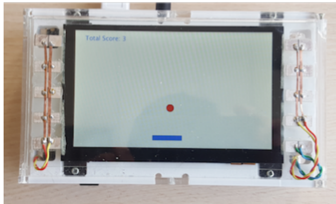
FIGURE 3.17: The setup of the pong game which enables visually impaired users to play. Two different kinds of textures can be perceived for each correct or wrong direction of sliding the blue paddle to get the red bouncing ball.
