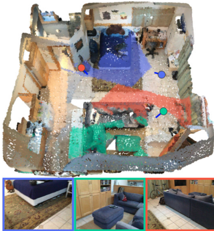
Figure 5.1 – Combining 2D and 3D Information. We propose to merge the complementary information between point clouds and a set of co-registered images. Using a simple visibility model, we can project 2D features onto the 3D points and use viewing conditions to select features from the most relevant images. We represent images at their position with the symbol \bullet and color the 3D points according to the image they are seen in.
