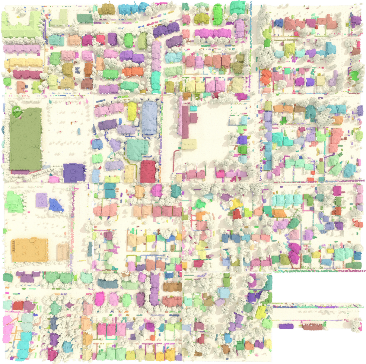
Figure 4.7 – Large-Scale Inference on DALES. Largest scan that SuperCluster can segment in one inference on an A40 GPU: 15.3 tiles, 7.8km 2 , 18.0m points, 589k superpoints, 1727 target objects, and 1559 predicted objects. Inference takes 10.1 seconds.
