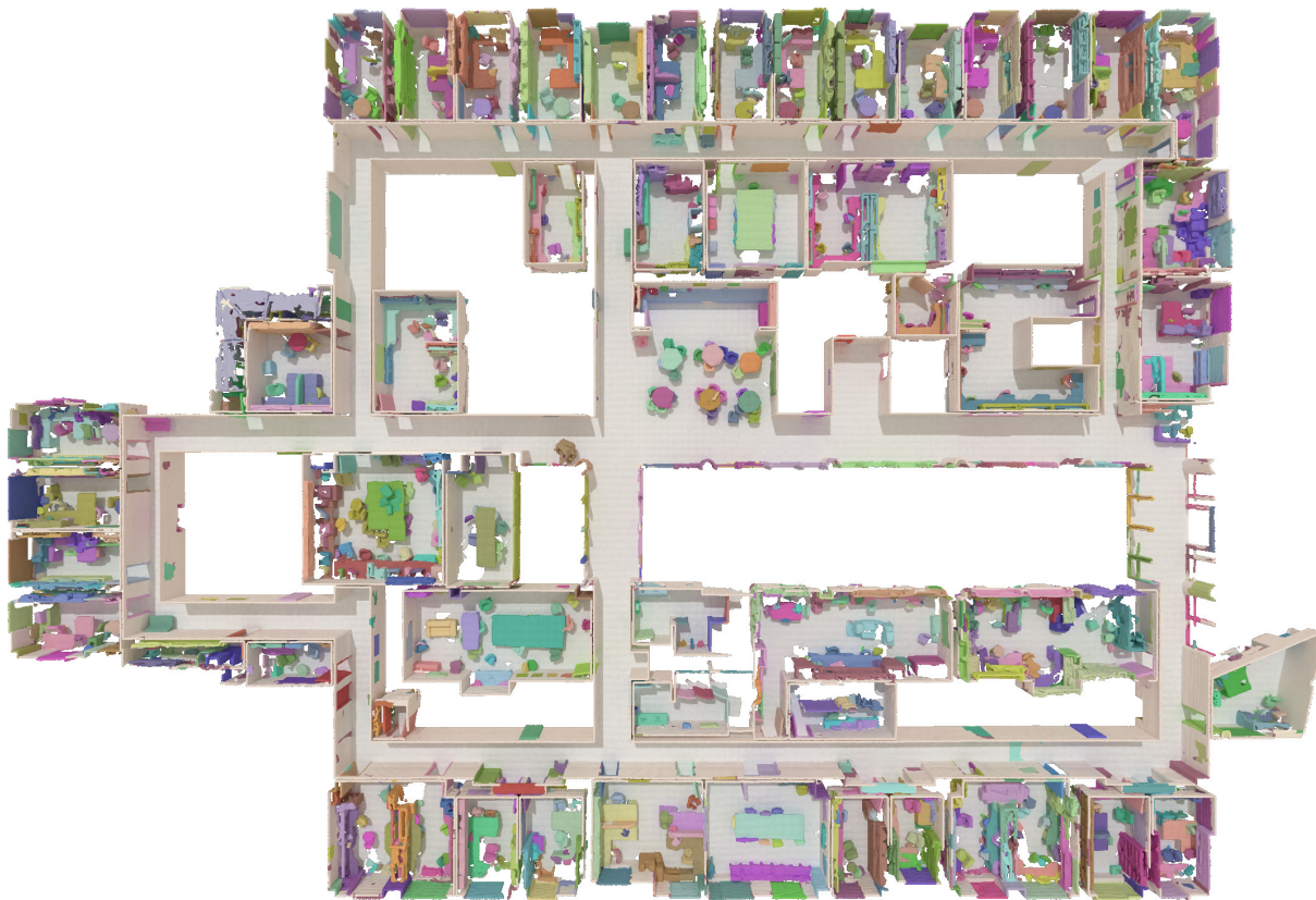
Figure 4.1 – Large-Scale Panoptic Segmentation. We present the results of Super-Cluster for the entire Area 5 of S3DIS [14] (ceiling removed for visualization) with 9.2M points (78M pre-subsampling) and 1863 true “things” objects. Our model can process such large scan in one inference on a single V100-32GB GPU in 3.3 seconds and reach a state-of-the-art PQ of 46.3.
