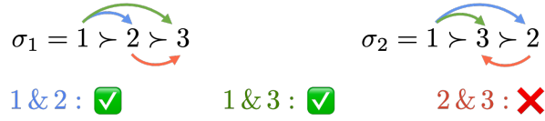
Figure 2.1: Illustration of the computation of Kendall tau distance. \sigma_1 and \sigma_2 agree that 1 \succ 2 and that 1 \succ 3 , but disagrees on items 2 and 3, because \sigma_1 orders 2 \succ 3 and \sigma_2 orders 3 \succ 2 . Therefore, the Kendall Tau distance between \sigma_1 and \sigma_2 is d_\tau(\sigma_1, \sigma_2) = 1 .
