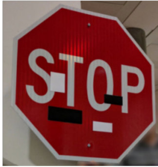
Figure 1.1: Adversarial attack against a real stop sign using black and white patches, from Eykholt et al. (2018) . The stop sign is misclassified by deep learning models as a 45 mph speed limit sign.
