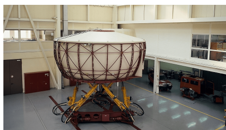
(a) Simulateur hybride Daimler-Chrysler [KH95]
