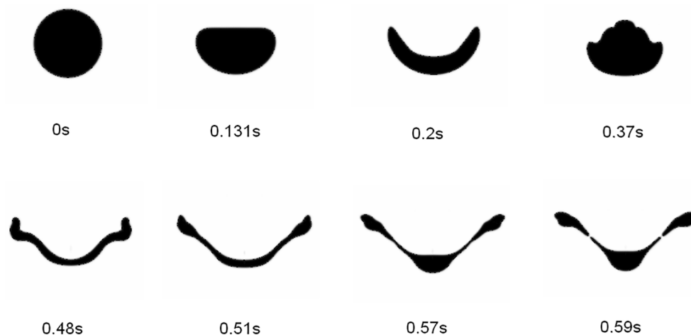
Fig. 7. Deformation and rim shear breakup of an iron drop within a magma ocean. In this model, Re = 92.4 , We = 20.3 , R_\mu = 100 (simulation #22 in Table 2).
