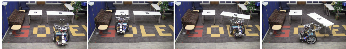
(A) Initial configuration. The goal is to reach the top right corner of the room. (B) Expected solution: push the square table; but it is stuck - constraint learned. (C) Expected solution: pull the long table; but it rotates unexpectedly because a wheel caster is locked - constraint learned. (D) Expected solution: rotate long table: rotated successfully and opening found.
