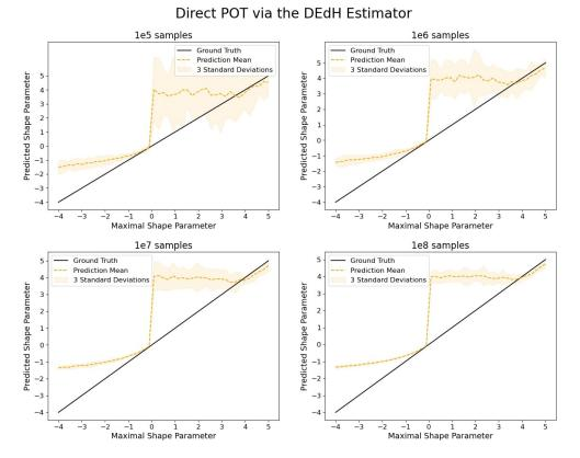
**Fig. C.10.:** Estimation of the shape parameter of the marginal by direct application of POT. We utilize the DEdH estimator as our estimator of choice.
