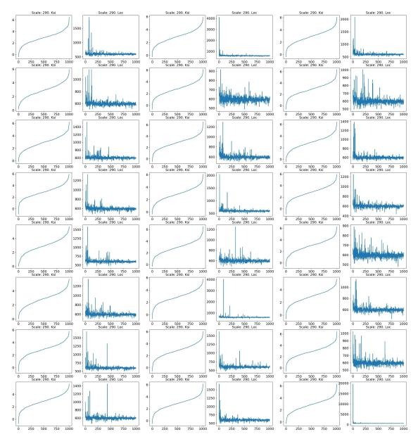
**Fig. C.8.:** We run 32 times the Gaussian Process experiment for length scale parameter value of 290. On each run, we calculate thresholds (sorted) of the 1000 conditional distributions determined by the 1000 choices of the training set, as well as their corresponding shape tail parameters. We see that higher thresholds correspond to lower shape parameters
