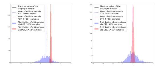
**Fig. C.2.:** Standard estimation of the shape parameter of the tails by simply applying the Pickands' Estimator, on average, gives poor results on fewer data (left). Cross tail estimation (CTE) gives the correct estimation on average. (right).
