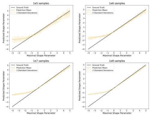
**Fig. C.9.:** In cases where the maximum tail shape parameter in the mixture of conditional distributions is positive, the estimated shape parameter of the marginal is also positive and equal to this maximal value. However, if this maximum value is negative, the estimated shape parameter is also negative. We utilize the DEdH estimator as our estimator of choice.
