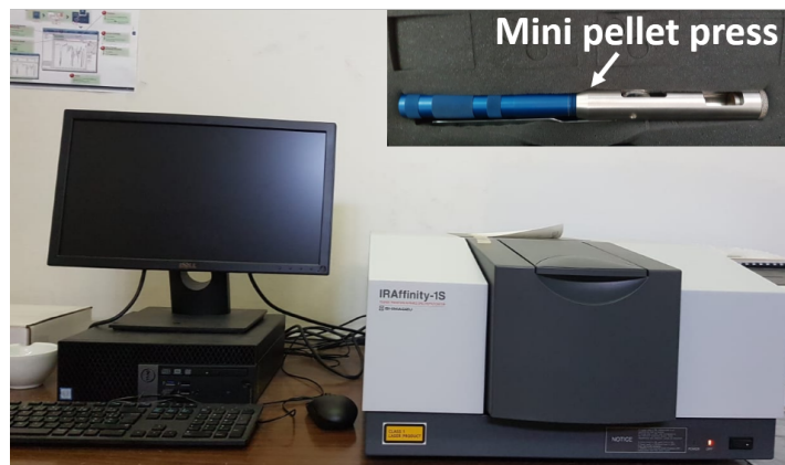
Figure 2.11: Images of the FTIR spectrophotometer and the mini press used for the preparation of high-quality pellets.
