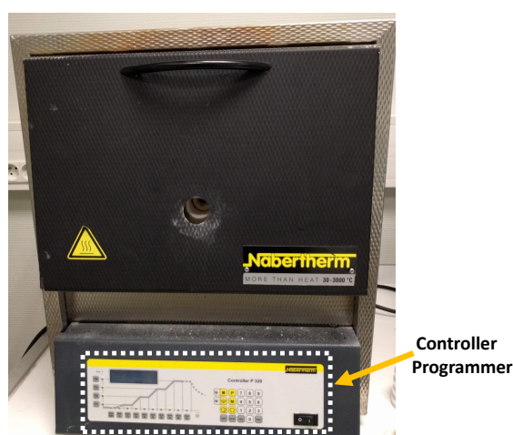
Figure 2.7: Image of the furnace used for the air annealing treatment of the samples.
