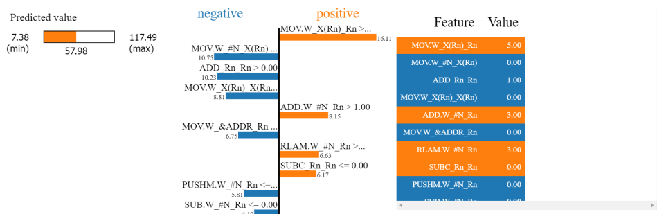
Figure 5.1 – Plot showing feature impacts on timing prediction for a basic block on MSP430.
