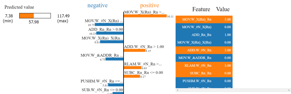
Figure 5.1 – Plot showing feature impacts on timing prediction for a basic block on MSP430.
