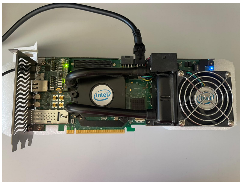
Figure 68 – The Stratix 10 GX development kit employed for evaluating the firmware comprising the neural networks.
