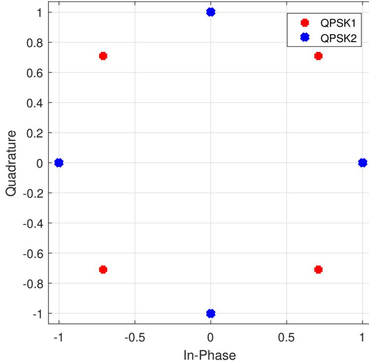
Figure 1.10: Constellation diagram for QPSK1 and QPSK2
