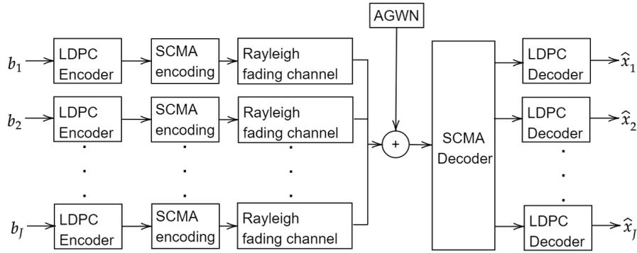
Figure 2.3:  $J$ -user LDPC encoded SCMA system
