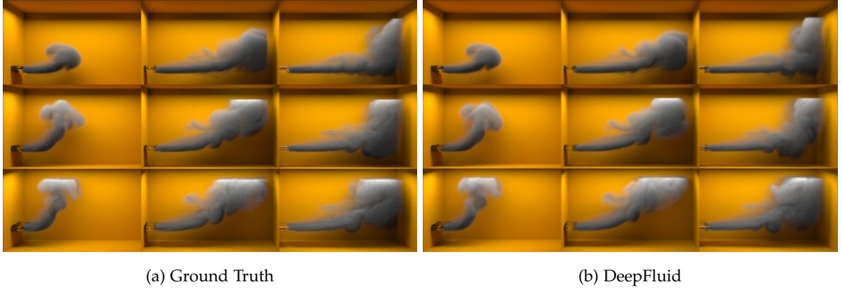
Figure 3.5: DeepFluid : Simulation results from Kim et al. (2019), where a CNN -based model is used to perform fluid simulations for computer graphics. The model is trained on simulations obtained with Mantaflow (Pffaff and Thuerey, 2016), a simulation software inspired by the Stable Fluid algorithm (Stam, 1999), a fast and stable yet not physically accurate algorithm for rendering fluids.
