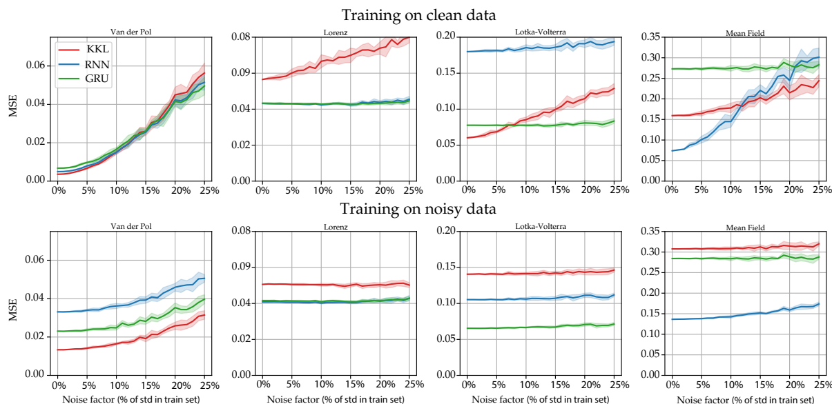
Figure 5.5: Evaluation on noisy setup – (Top line) Robustness against noisy inputs for models trained on perfect data. Deep-KKL shows limited success in handling the perturbation. (Bottom line) The models are trained with noisy measurements (added Gaussian noise with std. corresponding to 5% of the std. measured on the training dataset), which tend to improve robustness, but also degrade the performance.
