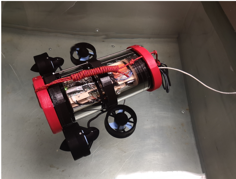
Figure 5.8 – Picture of PlaSMAR during one of the first pool tests. Configuration equivalent to RSM with four fixed thrusters.
