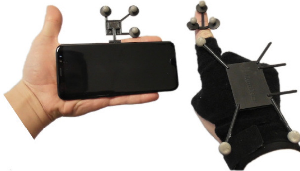
Figure 5.2: 3d printed markers on the smartphone and the user's dominant hand and the index finger.
