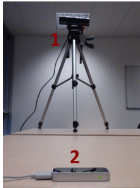
Figure 4.8: Sensor placement. 1. Kinect, 2. Leap Motion
