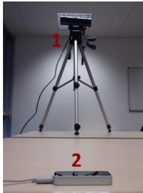
Figure 4.8: Sensor placement. 1. Kinect, 2. Leap Motion
