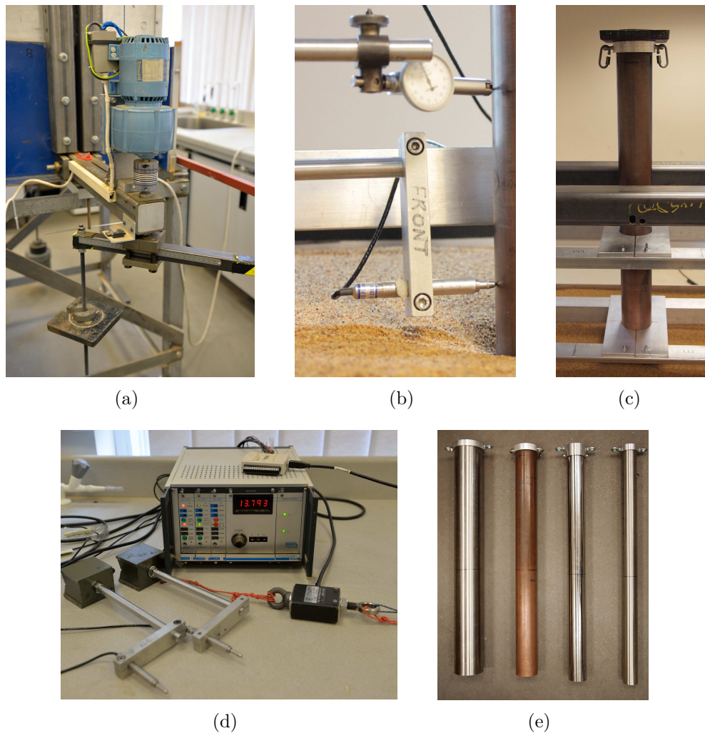
Figure 2.5: (a) Driving motor (b) LVDT and Dial Gauge (c) Pile during installation (d) Data acquisition system (e) Pictures of the piles used for testing
