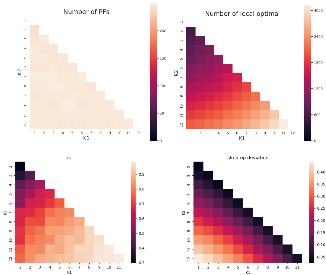
Figure 6.1: Additional Statistics computed over heterogeneous MNK landscapes of dimension 16. Number of Pareto fronts per instance, computed using the non-dominated sort algorithm 3 (top left). Average Number of local optima per instance (top right). Average Number of connected components (bottom left). Proportional deviation of single-objective local optima between each objectives (bottom right).
