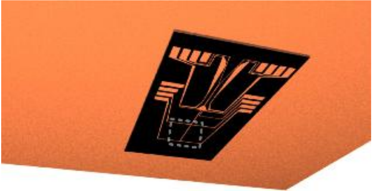
Figure 14. An atom chip [From Stickney (2007)]
