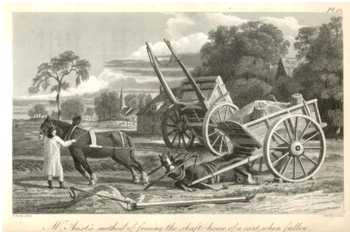
Illustration 89. W. Aust, « Machine for freeing the Shaft Horse, when fallen with a loaded Cart », Transactions of the Society , vol. 35, 1817. © RSA London
