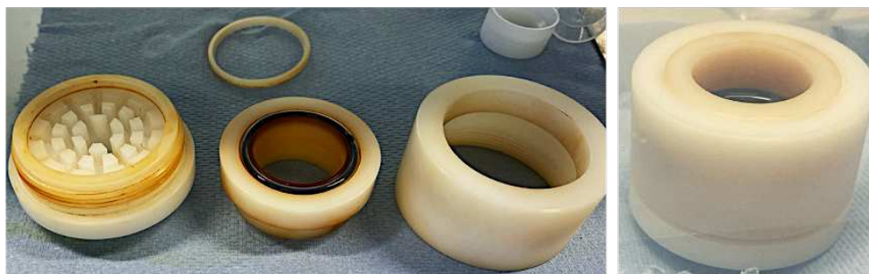
Figure S6.1 Ceramic interfacial polymerization setup, unassembled on the left and assembled on the right.
