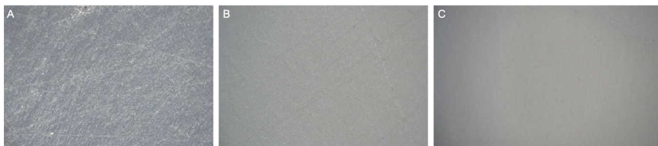
Figure 7.9 Stereo-microscopy for three different samples of the PA6 substrates after polishing according to Table 7.7 From left to right, Test 3 for F136 (A), Test 5 for FLE40 (B) and Test 7 for FLE40 (C).
