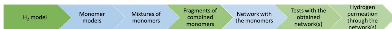
Figure 4.1 Modelling process to obtain hydrogen permeation in a dense polymer network of HCCP and Phg. The first step is detailed in Chapter 3 and the blue steps have been mainly carried out by another member of the project team.
