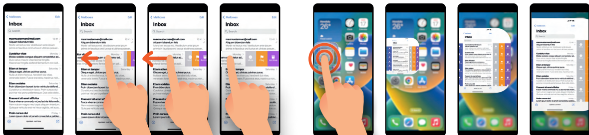
Figure 5.1 – Left: Example of a swipe-revealed widget, or Swhidget : a user swipes an email away from the edge of a touch screen to reveal hidden buttons. Right: We explore the potential of adding interaction hints in animated transitions to temporarily expose users to Swhidgets as a means to increase their discoverability.
