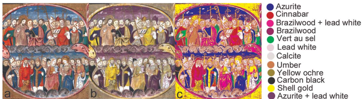
Fig. 1. “Assembly of Saints” (MAR_97): RGB (a) IRFC (b), and classification (c) images. The palette is rich and counts about 12 pigments and a many variation of tones.
