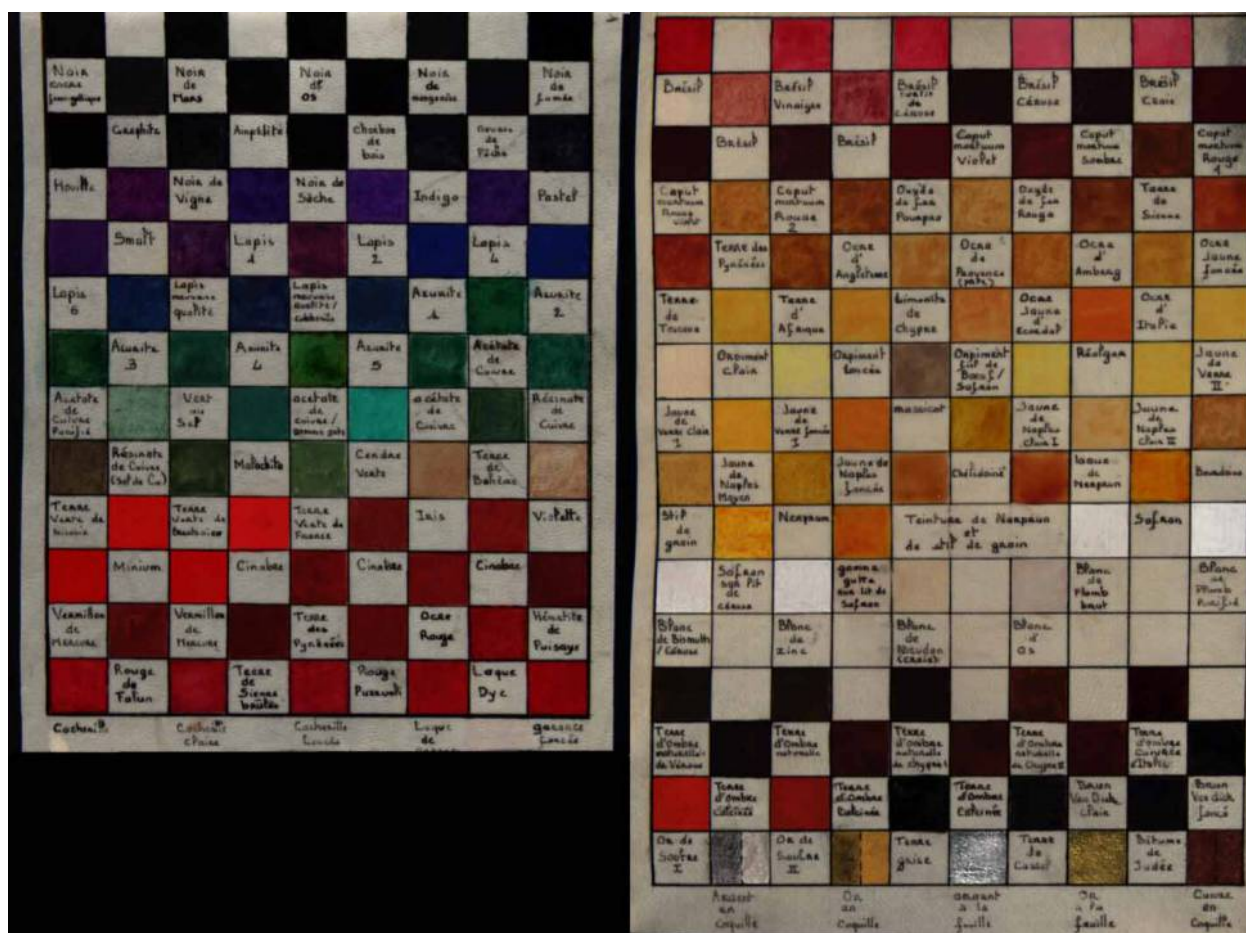
Figure 1 Charts of reference medieval pigments. Traditional medieval pigments have been prepared in accordance with medieval techniques by a specialist (Renaud Marlier) and are painted on parchment.
