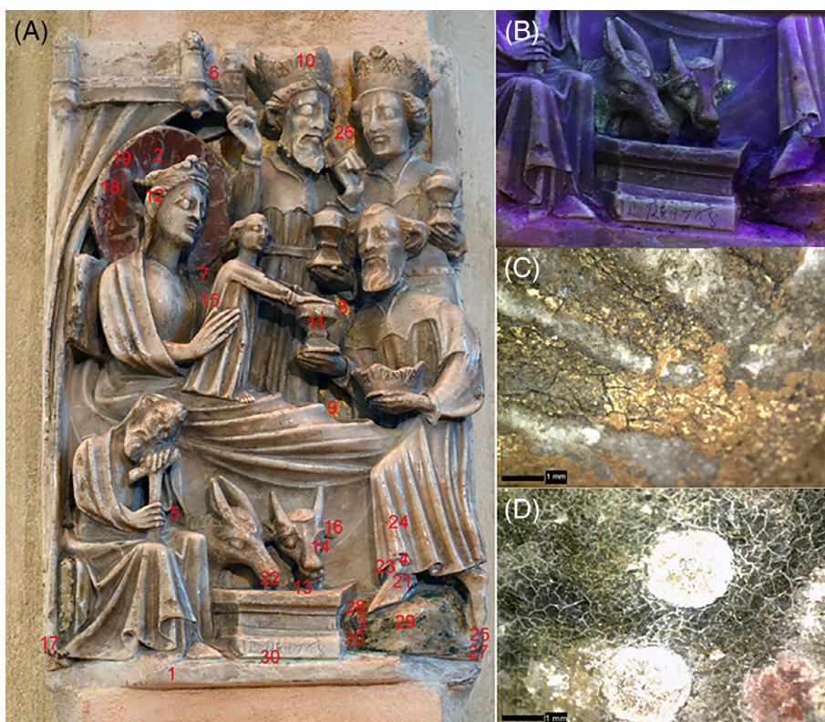
FIGURE 3 A, The Lormont's panel with the analysis points in red; (B) yellow fluorescence emission on the animals obtained under a UV light; (C) image of the Magi's gilded crown obtained by microscope x50; (D) "Daisy" on the green grass showing a network of cracks
