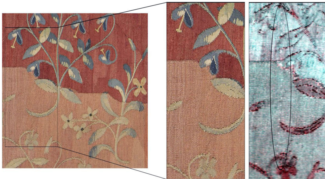
Fig. 4 On the left, detail on the bottom right of Mon seul désir tapestry (33 cm × 29 cm) ©Musée de Cluny. On the right, false colours hyperspectral image in the SWIR range ( R = 2205 nm; G = 1575 nm; B = 1536 nm)
