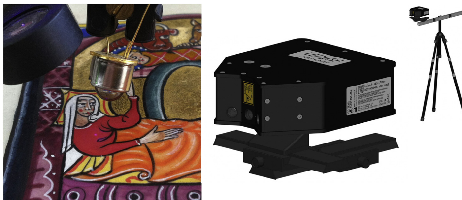
Fig. 1. 375 nm LED in action with our lab prototype on a facsimile reproduced in accordance with the medieval techniques. The analytical head of the LED \mu SF device built by the manufacturer Erma Electronique. The head is finely positioned by means of a micrometric X-Y stage in particular to adjust the working distance and the analyzed spot. The system supported by a tripod for in situ analysis.
