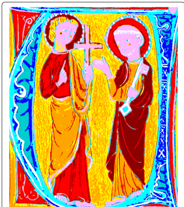
Figure 9 Mapping (classification) of the pigments based on spectra comparison: dark blue color corresponds to "azurite", turquoise blue to "lapis lazuli", dark red to "cinnabar", bright red to "cochineal on cinnabar", dark yellow to "orpiment" and pale pink to "white lead".
