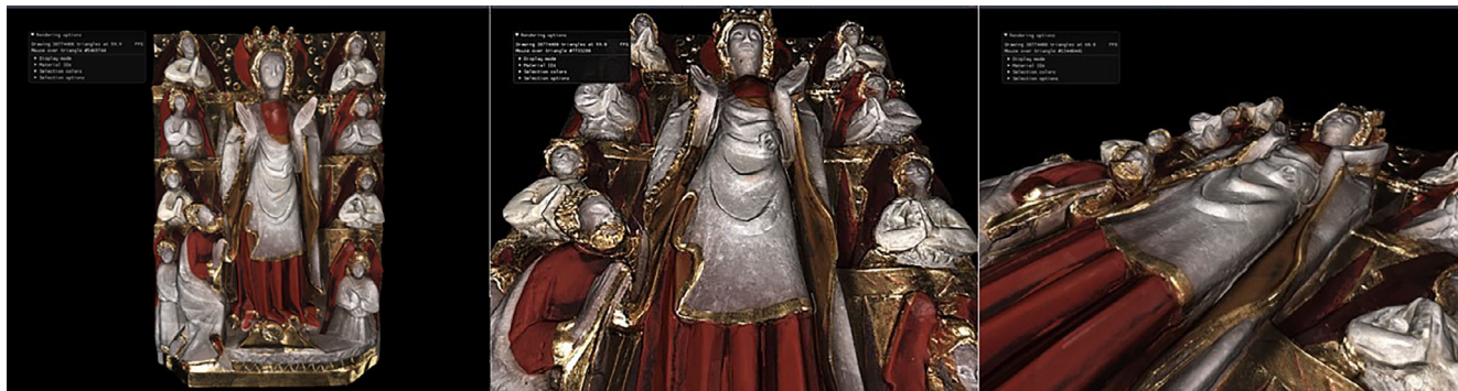
FIGURE 8 Digital reconstruction of the alabaster manufactured by A. Bély and M. Mulliez. The presented model contains 40 million triangles and with one colour per vertex. To generate the model, 30 000 of high dynamic range images were acquired
