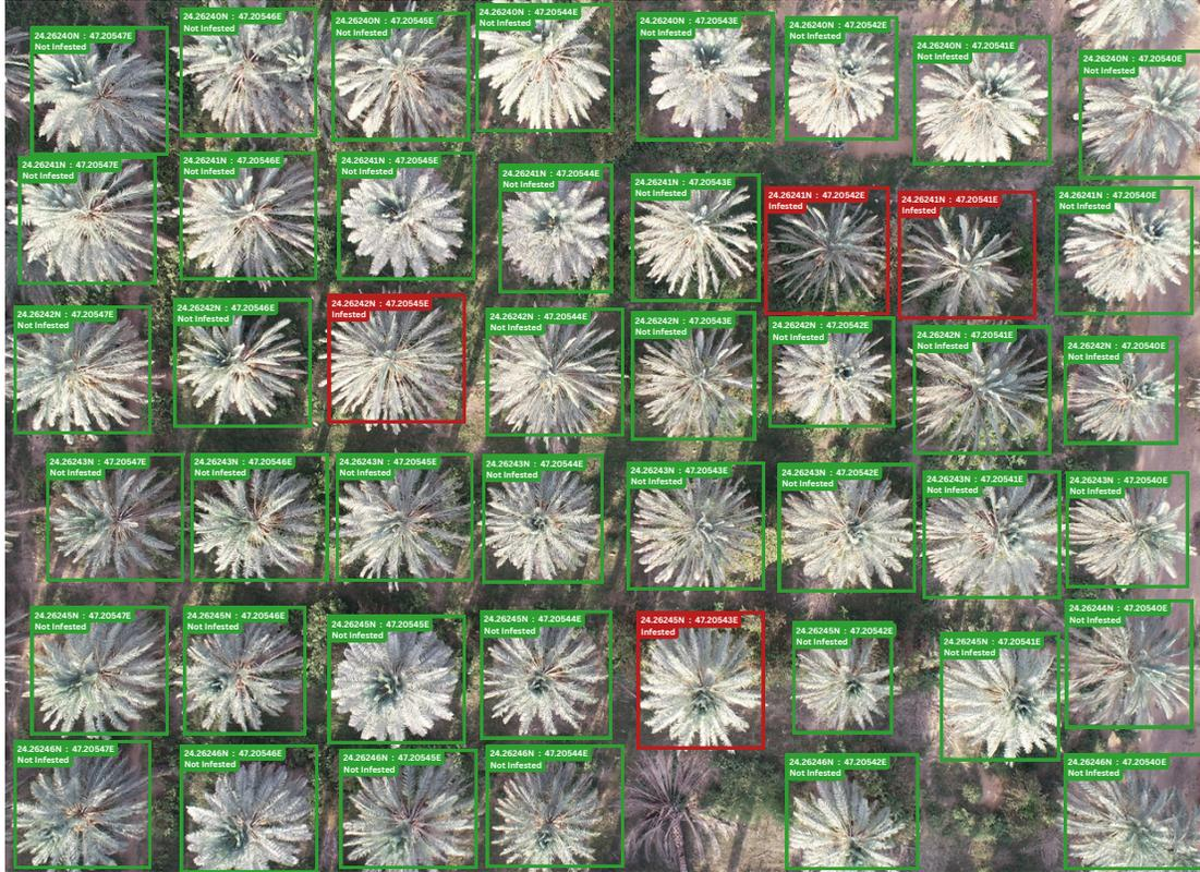
FIGURE 6.11: RPW Map Visualizing Infested and Not Infested Palm Trees.
