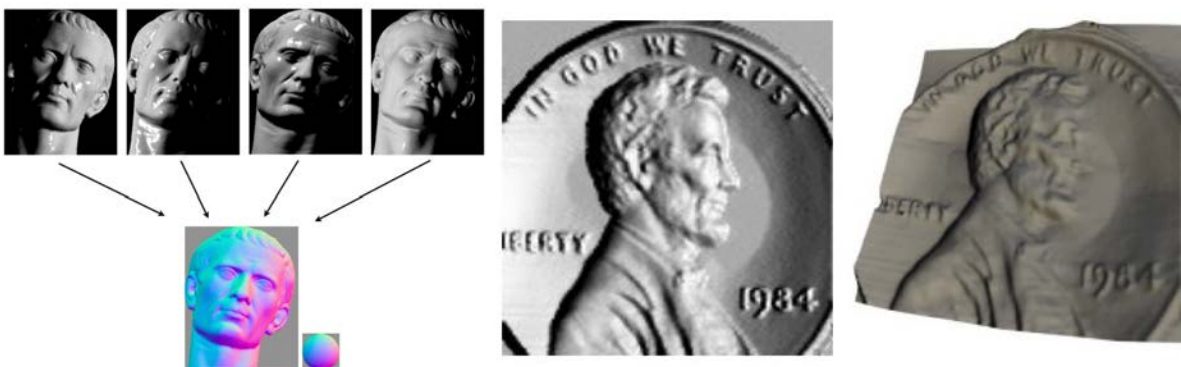
Figure 1.3: Illustration of the principle of shape-from-shading and application to a coin. Images taken from [94]
