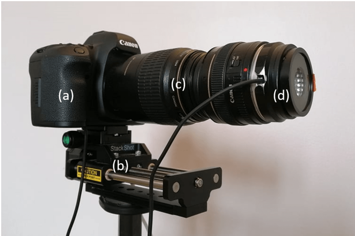
Figure 1.16: Used acquisition device. (a) Canon EOS 5D II camera; (b) motorized rail; (c) optical system using a 100mm lens and an inverted 50mm lens; (d) light ring with diffuse filter.
