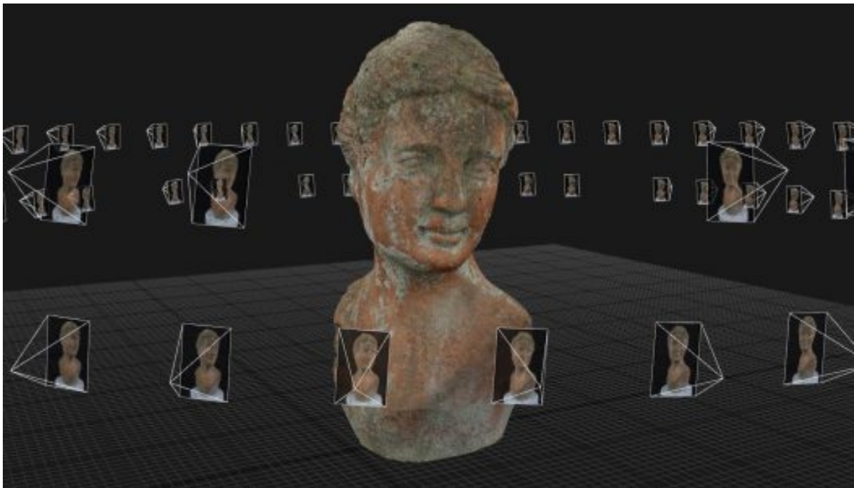
Figure 1.4: Image taken from RealityCapture Software by the website 3D Scan Expert . Illustration of the 3D object acquired and the positions get by SfM for each camera.
