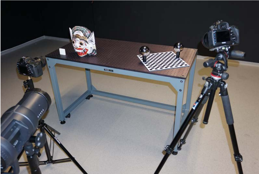
Figure 3.13: Set-up acquisition in laboratory. Example of the acquisition of a Balinese mask.
