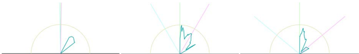
Figure 3.27: Polar plots of the golden material of the Balinese mask with \theta_i = 1^\circ , \theta_i = 30^\circ and \theta_i = 50^\circ .
