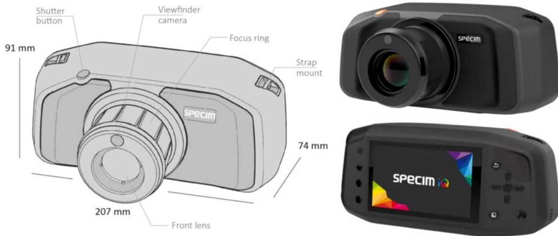
Figure 2.3: Vectorial visualization of the Specim IQ with annotations and dimensions on (left) and commercial pictures (right). Figure taken from [25].
