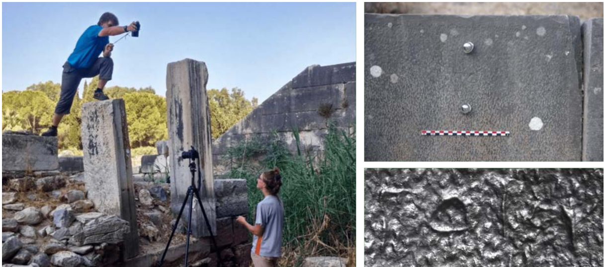
Figure 3.9: Pictures illustrating the RTI method. Left: RTI shooting on Christian monograms. Top right: Photograph of a hyposthèneion of the theater of Miletus: traces of a graffiti. Top left: Snapshot of the hyposthèneion using the RTI software for specular enhancement in order to read a graffiti. Images taken from [41].
