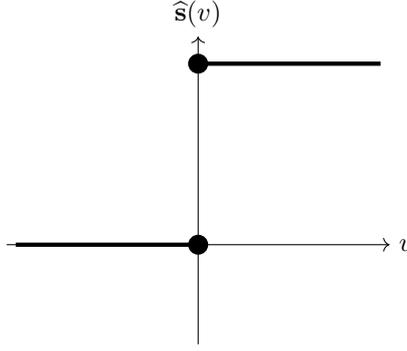
Figure 4.3: Krasovskii regularization of the step function  $\widehat{\mathbf{s}}(v)$ .
