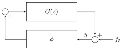
Figure 2.6: Feedback representation of a Lurie system is here used to represent PWA systems. In this part,  $\phi$  will be a vector of ramp functions. The term  $f_5$  is a constant vector that is added to the output of the linear block  $G(z)$  to generate the input  $y$  of the nonlinearity  $\phi$ .
