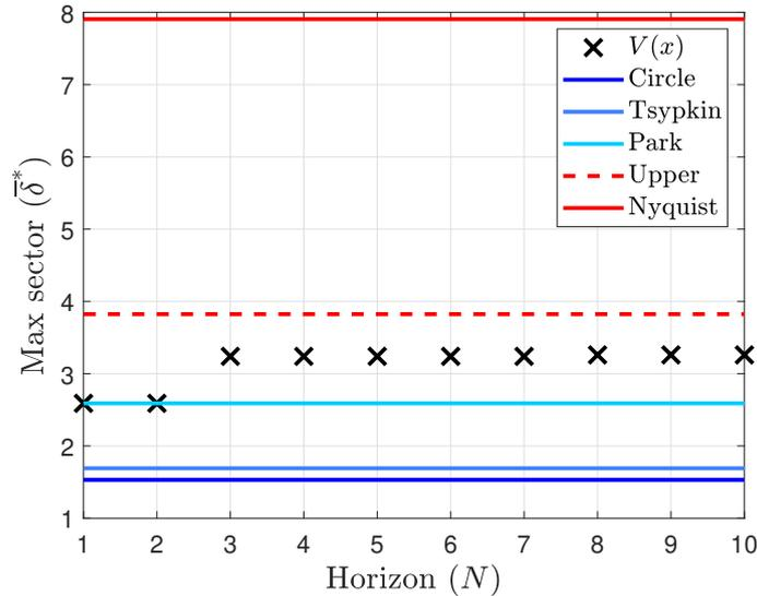
Figure 2.3: Maximum sector  $\delta$  obtained by Proposition 2.1 for  $G_4(z)$  as a function of the horizon  $N \in [1, 10]$ . We also plot the bounds achieved using the Circle criterion, the Tsyarkin Lyapunov function and the function from [132]. The upper limit set by the Nyquist gain is also plotted.
