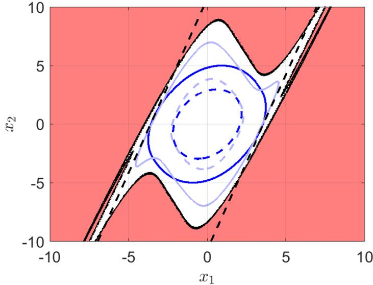
Figure 2.4: Regional stability of the second numerical example. Positive invariant sets of the Lyapunov function  $V(x)$  from (2.5) are shown in blue, with blue dashed lines corresponding to sub-level sets. Light blue corresponds to  $N = 4$  and dark blue to  $N = 1$ . Black dashed lines denote the limits  $\{x : \nu_0(x) = \bar{y}, \nu_0(x) = \underline{y}\}$ . Initial conditions from the red region did not converge to the origin.
