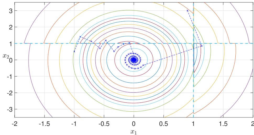
Figure 4.10: Trajectories for the system along with the partitioning of the state space introduced in (4.30). Initial conditions are selected as  $(0.9, 3)$ ,  $(-1, 0.5)$ . Note that the level sets of the computed Lyapunov function are disconnected. These disconnected sets appear, for instance in the set  $\{x \mid x_1 \geq 1, x_2 \leq 1\}$  close to the point  $(1, 1)$ .
