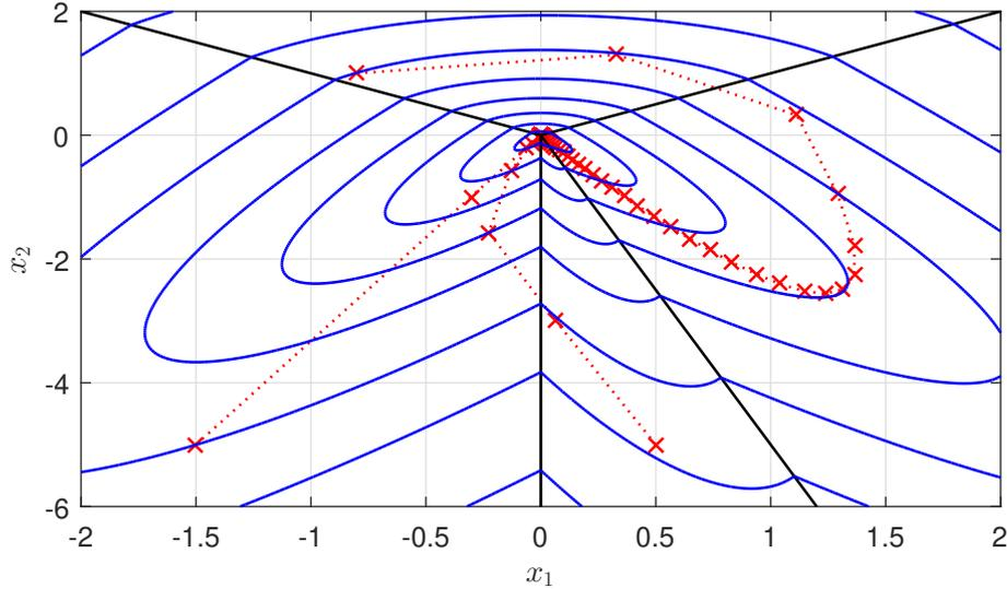
Figure 3.4: System trajectories and Lyapunov function level sets for Example I.
