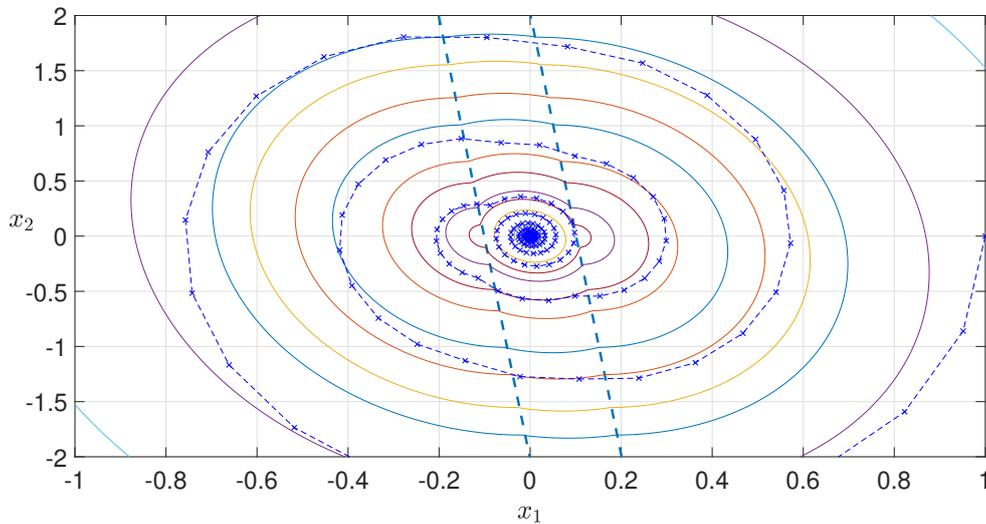
Figure 4.7: Simulations in Example 4.4.1. Level sets of the function  $W(x) = \max V(x)$  and the trajectory  $\sigma$  of (4.29) starting from  $(1, 0)$  (dashed-crossed line). The dashed line indicates the set where  $Kx + d = 0$ , namely, the set where the argument of the ramp function and the step function is equal to zero.
