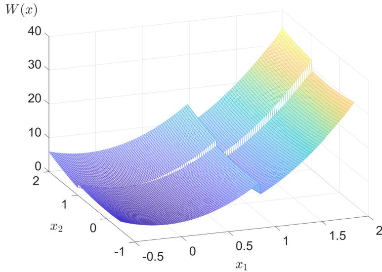
Figure 4.9: Lyapunov function  $W(x)$  for Example 4.4.3.
