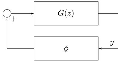
Figure 2.1: Feedback representation of a Lurie system.
