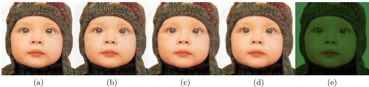
Figure 1.1 – Examples of measurements for different image inverse problems: (a) the original image baby.png of the Set5 dataset [22], (b) image corrupted with a Gaussian noise with a standard deviation \sigma = 20 , (c) blurred image with a gaussian kernel of size 5 \times 5 with a standard deviation \sigma = 20 , (d) down-sampled and then upsampled image with a magnification factor of 4 and using a bilinear interpolation, (e) mosaic image obtained using the Bayer kernel.
