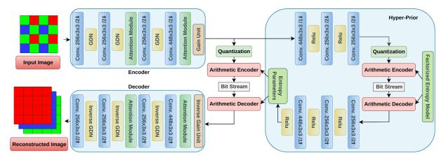
Figure 5.1 – Joint compression-demosaicking architecture with raw data as input.
