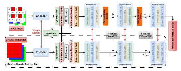
Figure 5.4 – Joint compression-demosaicking architecture with a guiding branch.
