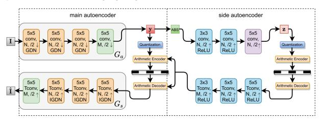
Figure 4.6 – Joint compression and denoising architecture. Source: [Alves de Oliveira et al., 2022].
