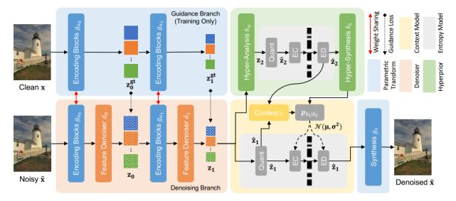
Figure 4.7 – Two-branch design for a joint compression and denoising network trained with pairs of ground truth and noisy images. Source: [K. L. Cheng et al., 2022]
