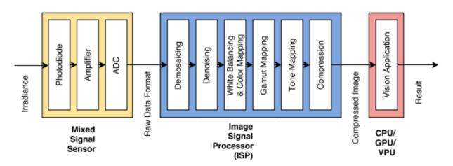
Figure 4.5 – Standard image processing pipeline. Source: [Buckler et al., 2017].
