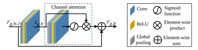
Figure 5.5 – Residual channel attention block (RCAB). Source: [Y. Zhang et al., 2018].
