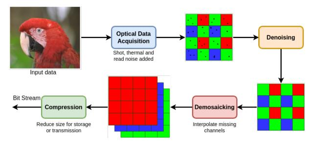
Figure 4.1 – Simplified imaging processing pipeline.
