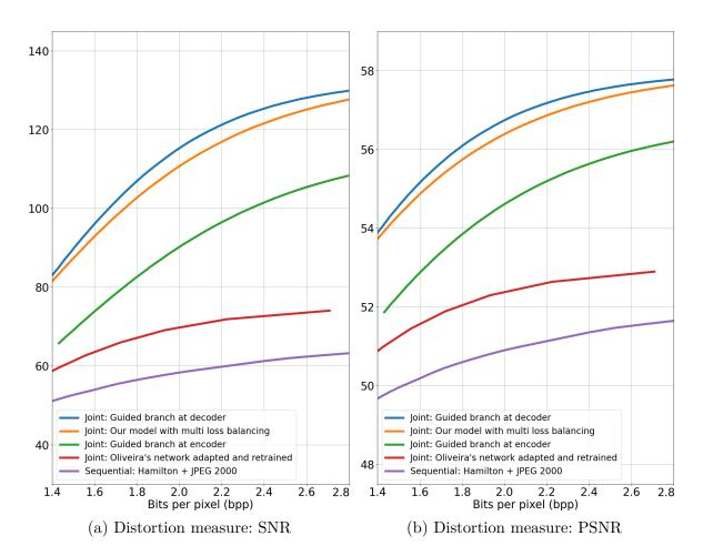
Figure 5.6 – Study of the position of the guiding branch in joint demosaicknig and compression architecture.
