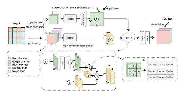
Figure 4.4 – Self-guidance architecture. Source: [L. Liu et al., 2020].
