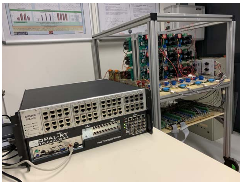
Figure 5.14: LAPLACE-MMC global view with and its connection to the OP5600.
