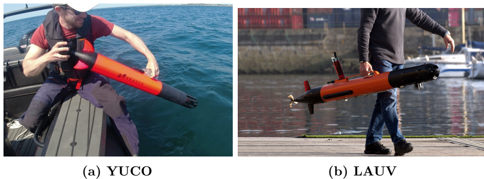
Figure 1.11 – AUV YUCO et LAUV
