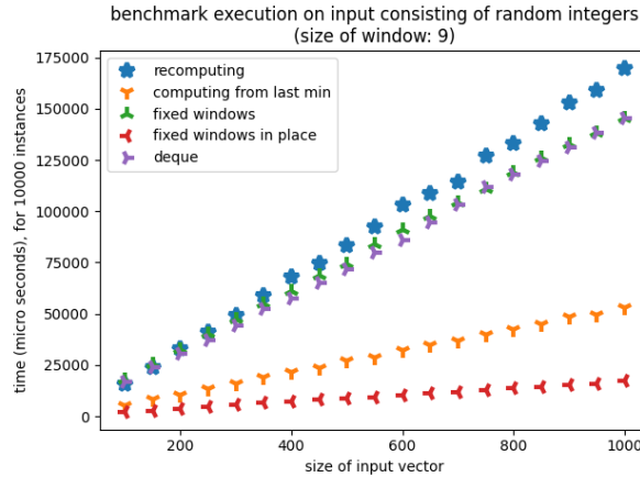
Figure 4.6: Comparison of five approaches for computing sliding window minimum. The input vector is composed of random integers. The size of the window is set to 9 and for each size of the input vector, 10000 instances were tested.
