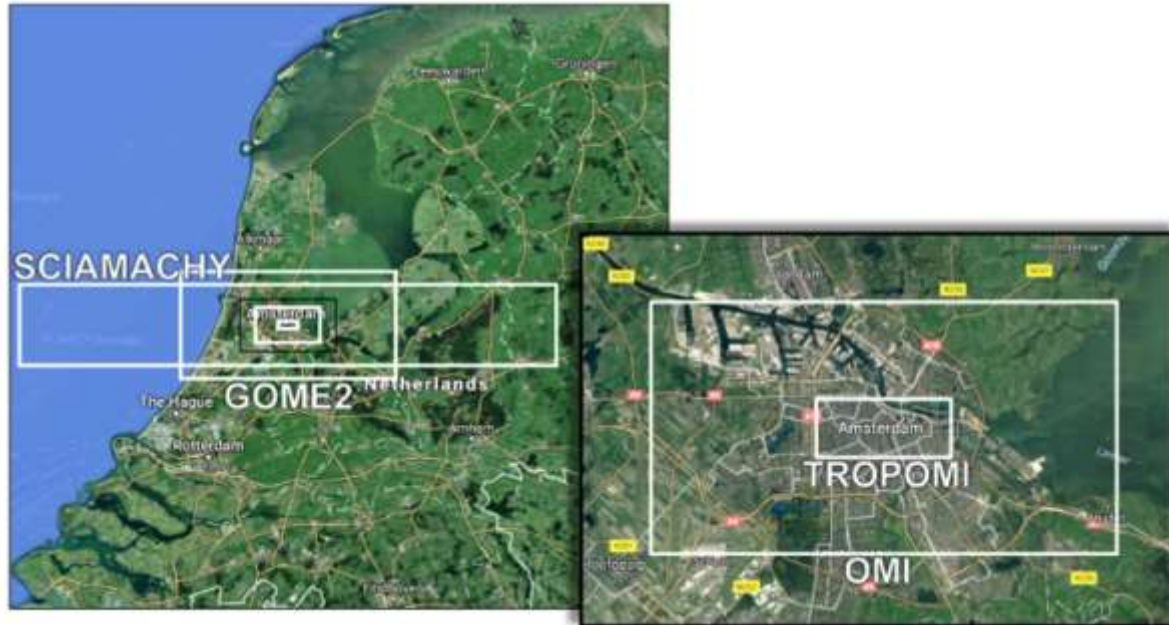
Figure 26 Spatial resolution comparison of satellite instruments. Note that TROPOMI pixel size further decreased now (Taken from BIRA-IASB, www.aeronomie.be/en/news/2021/three-years-tropomi-measurements )
