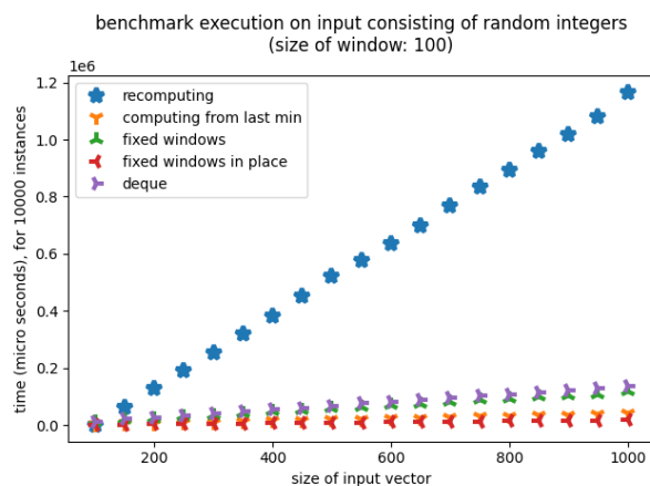
Figure 4.7: Comparison between 5 approaches for computing sliding window minimum. The input vector is composed of random integers. The size of the window is set to 100.
