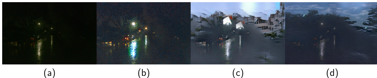
Figure 4.9: Style transfer and data augmentation methods with from left to right: Fig. 4.9a The input image, Fig. 4.9b CoMoGAN [Pizzati et al. 2021], Fig. 4.9c ManiFest [Pizzati et al. 2022], Fig. 4.9d MUNIT [Huang et al. 2018] trained on the Waymo dataset. These style transfer methods do not preserve the integrity of the scene in the input image and add hallucinations.
