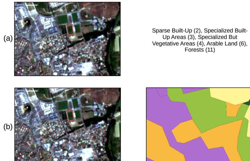
Figure 2.2 – Difference between scene classification (a) and semantic segmentation (b). Reference data has been taken from Wenger et al. [2022a]. Legend is also in the paper.
