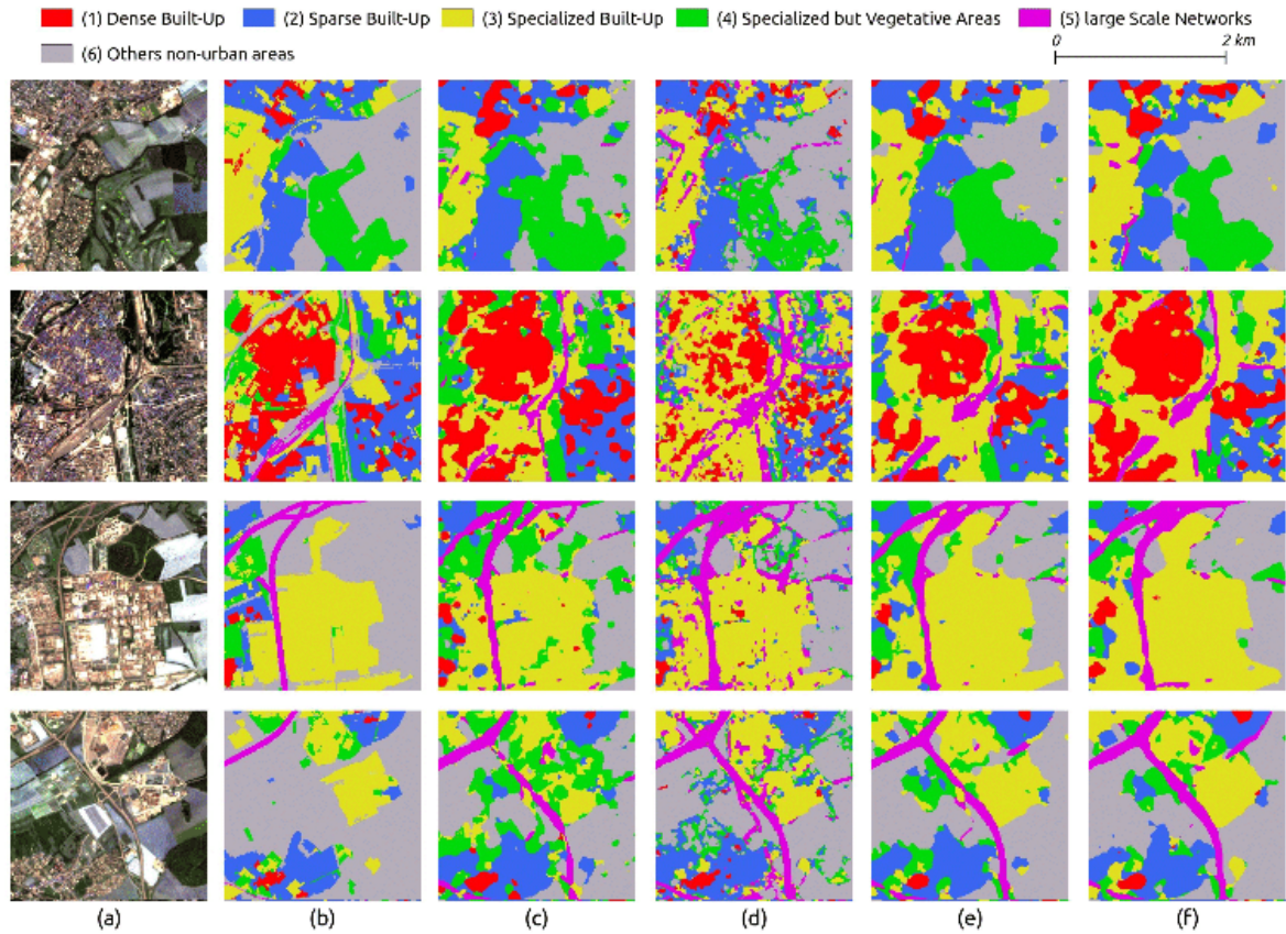
Figure 4.9 – Semantic segmentation results for test zone over Metz. (a) and (b) represent subset image and reference data respectively, (c) and (d) are respectively U-Net-IRRG and U-Net-Index and (e) and (f) are U-Net-Encoder and U-Net-Decoder.
