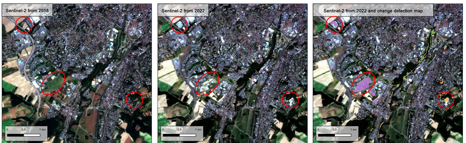
Figure 6.10 – Change detection near Mulhouse (subset 3 maps the class to which the surfaces have changed).
