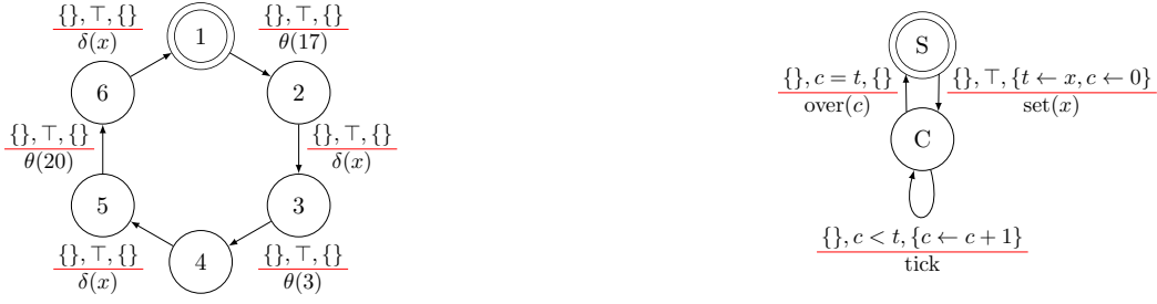
Figure 5.2: (a) An example of controller component (b) An example of counter component
