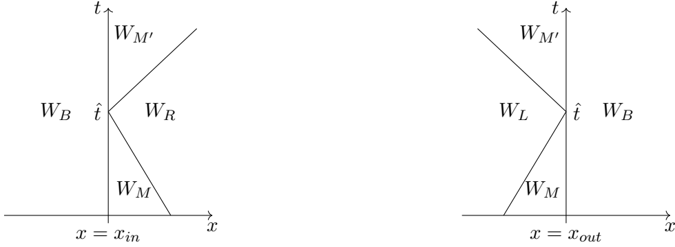
(a) Illustration of the states and the corresponding interacting waves at the left boundary (B.L).
