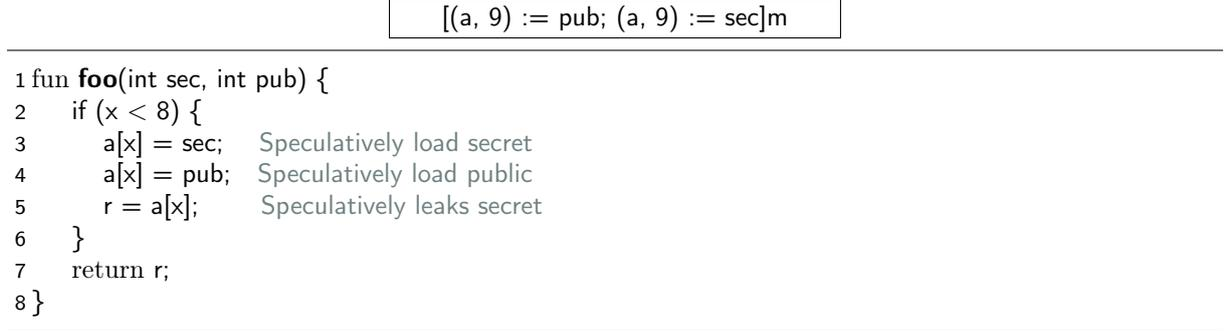
Figure 5.2 – Spectre-PHT attack
