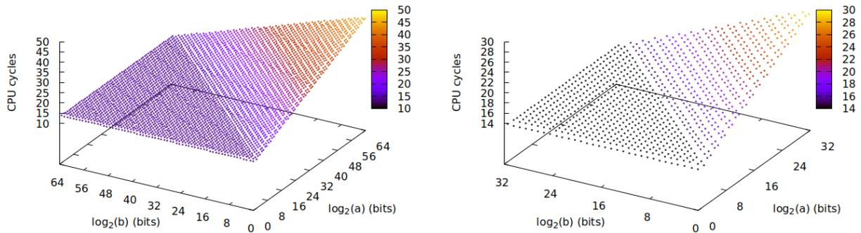
Figure 3.2 – Timing behavior of the `div` instruction on an x86 microprocessor (AMD EPYC 7F52) with 64-bit (left) and 32-bit (right) operands. It computes at once both quotient and modulo of its arguments  $a$  and  $b$ . Different microprocessor models exhibit different timing profiles.
