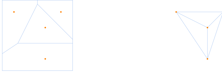
(a) Voronoi-diagram of random initial data in 2D. (b) Corresponding Delaunay-diagram, it is the dual graph.
