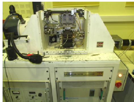
Figure 43: (a) Diagram and (b) photograph of the specific fretting apparatus.
