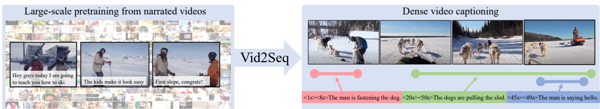
Figure 6.1: Vid2Seq is a visual language model that predicts dense event captions together with their temporal grounding in the video by generating a single sequence of tokens (right). This ability is enabled by large-scale pretraining on unlabeled narrated videos (left).
